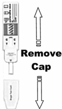
1. Bring the pouch to room temperature before opening it. Remove the test panel from the sealed pouch and use it as soon as possible.
